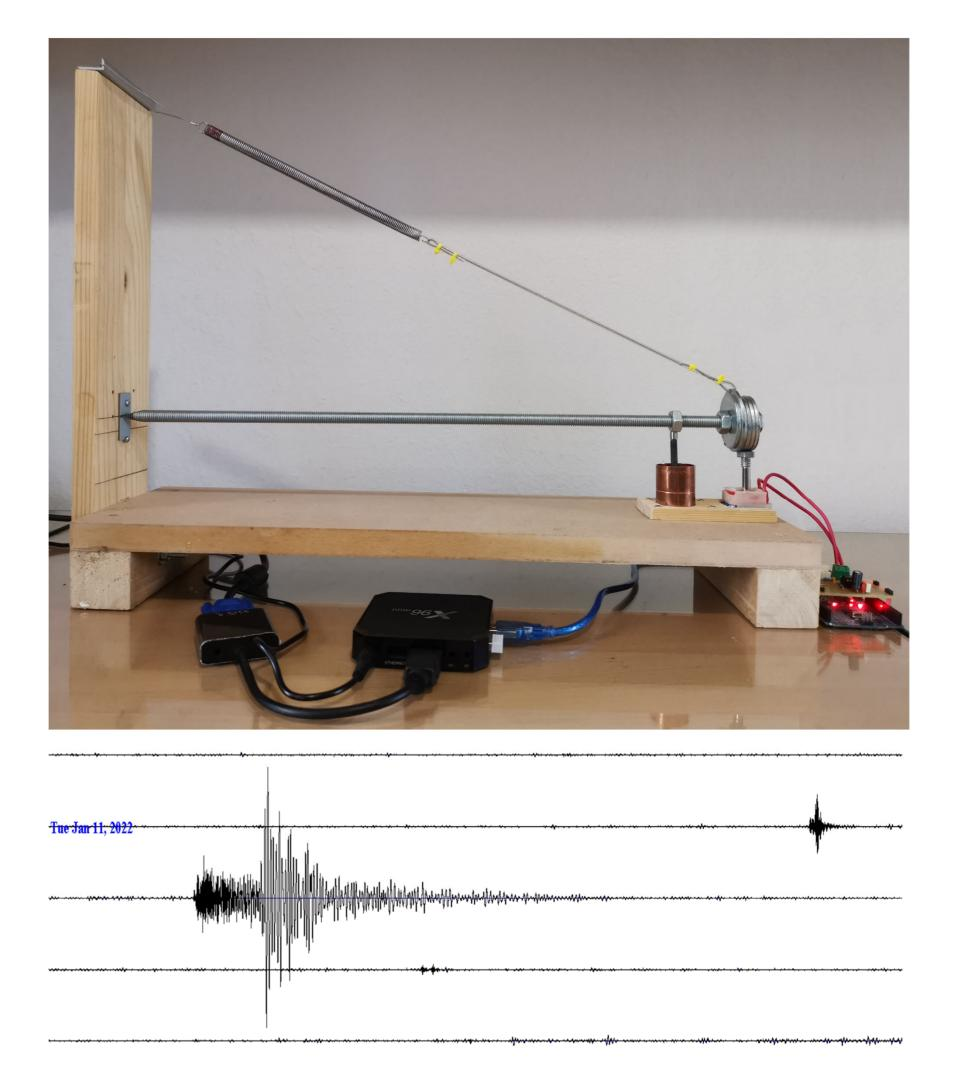
The ground-motion detection sensor is a mass-spring system combined with suitable electromagnetic and electronic devices to convert ground vibrations into electrical signals.
